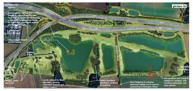
*Figure 5.* Borrow pit no. 1 (a – before exploitation, b – borrow pit design) (Highways England 2015)
