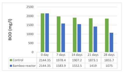
Figure 4. Retention period for BOD removal
