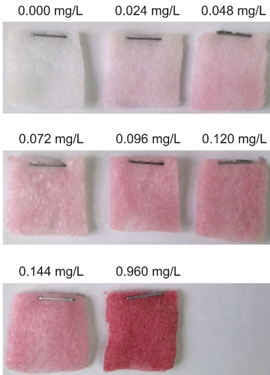
Figure 6. Examples of magnetically responsive, chitosan modified textile squares after azorubine extraction from water solution (100 mL; concentrations of the original solutions are shown) (reproduced from Safarik et al. 2019)
