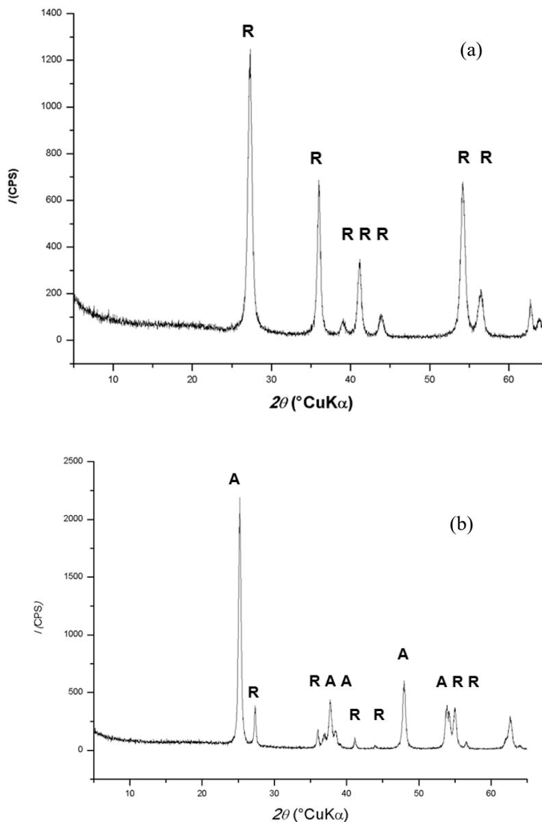
**Figure 2.** XRD spectra of N-TiO<sub>2</sub> (a) and UVC-TiO<sub>2</sub> (b)**Table 3.** Textural properties of powder catalysts determined using the nitrogen adsorption/desorption analysis
