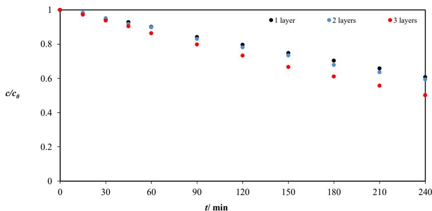
**Figure 8.** Influence of the number of layers of UVC-TiO<sub>2</sub> impregnated on glass vowing fibre on the degradation of imidacloprid
