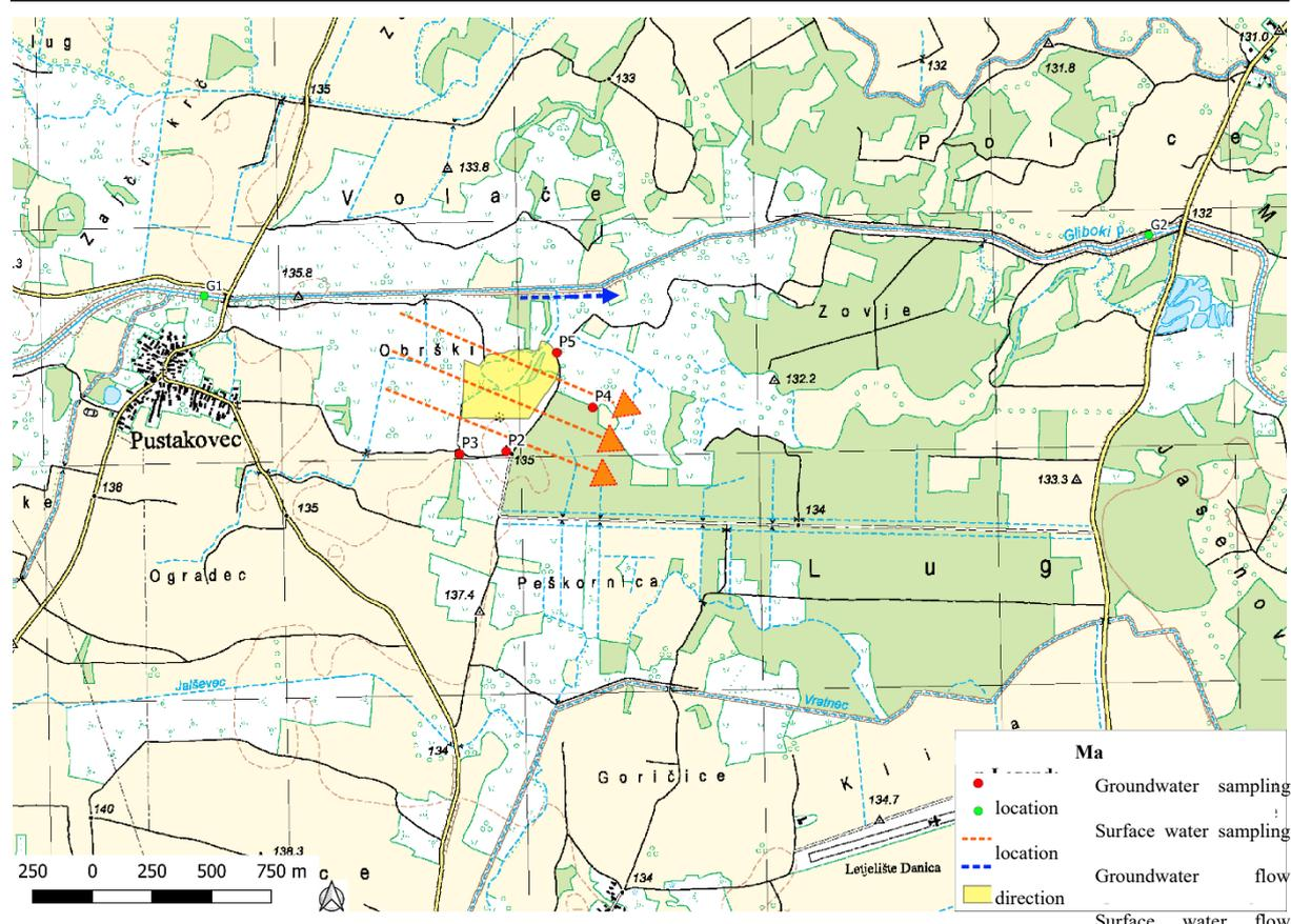
**Figure 2.** Piezometer locations and sampling points of the Gliboki water body (measuring profile G1 upstream) and measuring profile G2 downstream from the landfill which are marked with the flow directions of groundwater and surface water in the area of the Piškornica landfill (Source: Ruk, D. et al. (2018))
