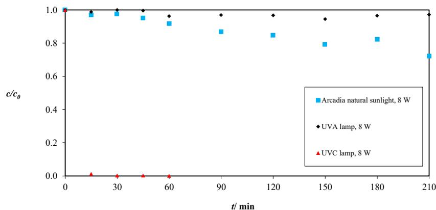
**Figure 4.** Photolytic degradation of imidacloprid using different irradiation source
