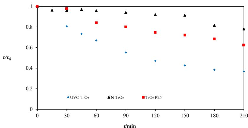
**Figure 5.** Comparison of three TiO<sub>2</sub> catalysts in the suspended form at the same reaction conditions
