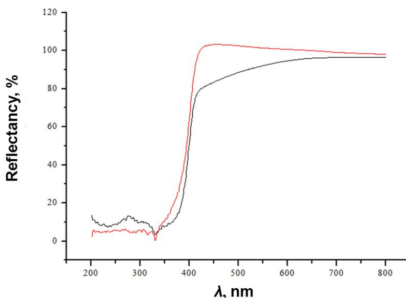
**Figure 1.** Diffuse reflectance spectra of N-TiO<sub>2</sub> (black line) and UVC-TiO<sub>2</sub> (red line)
