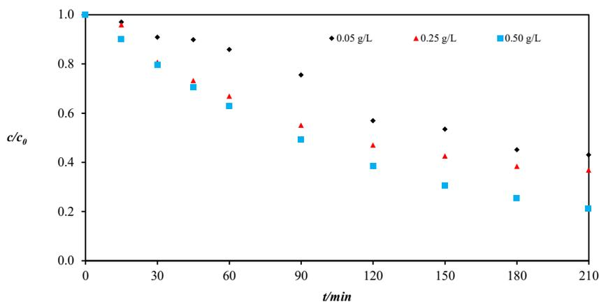
**Figure 6.** Influence of the concentration of UVC-TiO<sub>2</sub> on the degradation of imidacloprid
